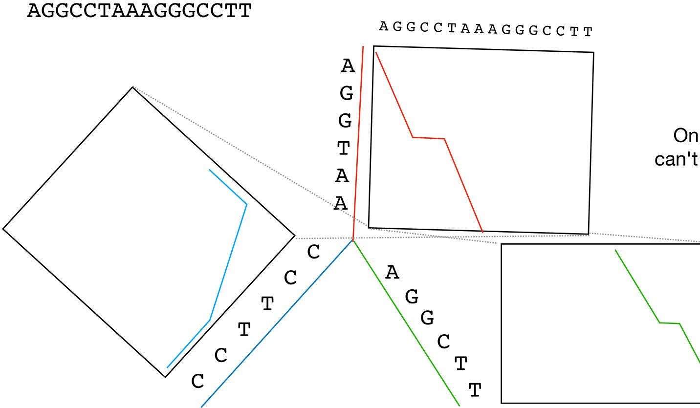
Only need to go to a depth of 2m since the best alignment can't be worse than deleting one string and inserting the other.
